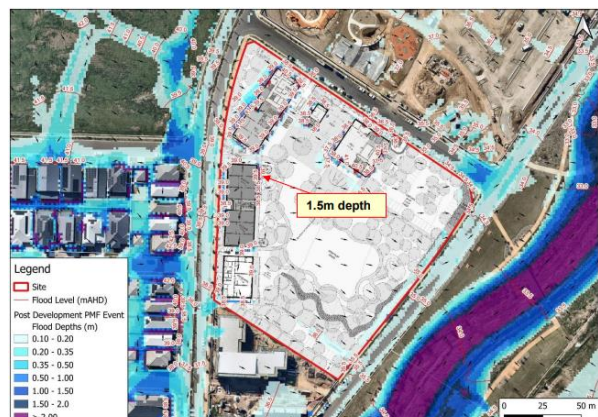
Figure 22 Peak flood levels and depths in the PMF event, post-construction
