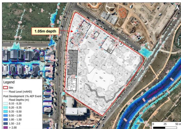
Figure 21 Peak flood levels and depths in the 1% AEP event post-construction
